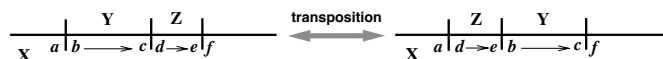
Fig. 4. A transposition operation. The operation breaks adjacencies (a, d), (c, b), and (e, f), and rejoins three pairs of free ends into (a, b), (e, d), and (c, f).
